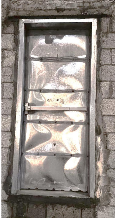
Figure 11: Unexposed face after the application of the hose stream
