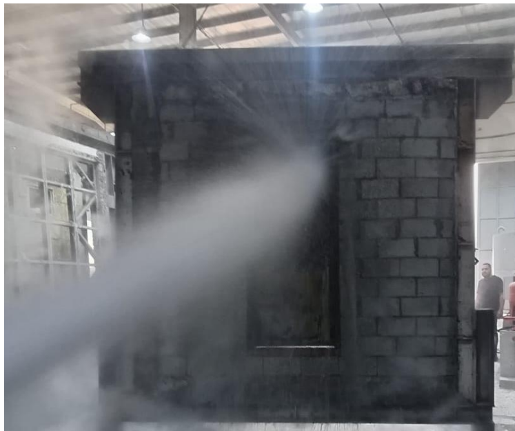
Figure 7: Hose stream test after 150 minutes fire endurance
