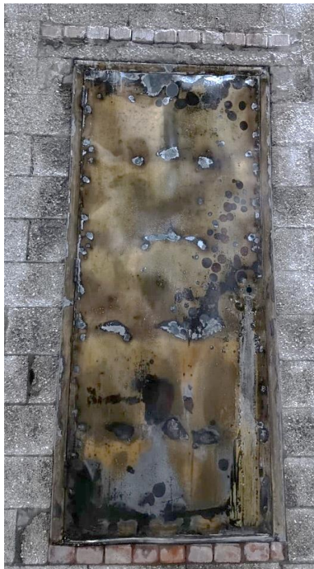
Figure 10: Exposed face After the application of the hose stream
