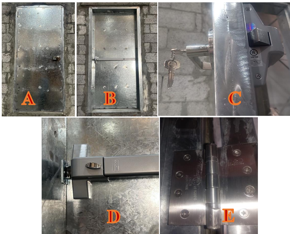
Figure 1: Photos of the door assembly and hardware, (A) Exposed face, (B) Un-Exposed face, (C) Latch bolt, (D) panic bar, and (E) Hinge
